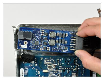
• Lift the DC to DC board out of the rear case.
