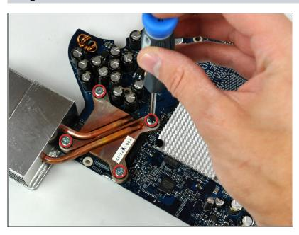
It may be necessary to hold the Phillips head screw sockets with a Phillips screwdriver while unscrewing the four Torx screws near the corners of the processor.
