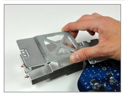
Lift the heat sink bracket up off the heat sink and the logic board.
