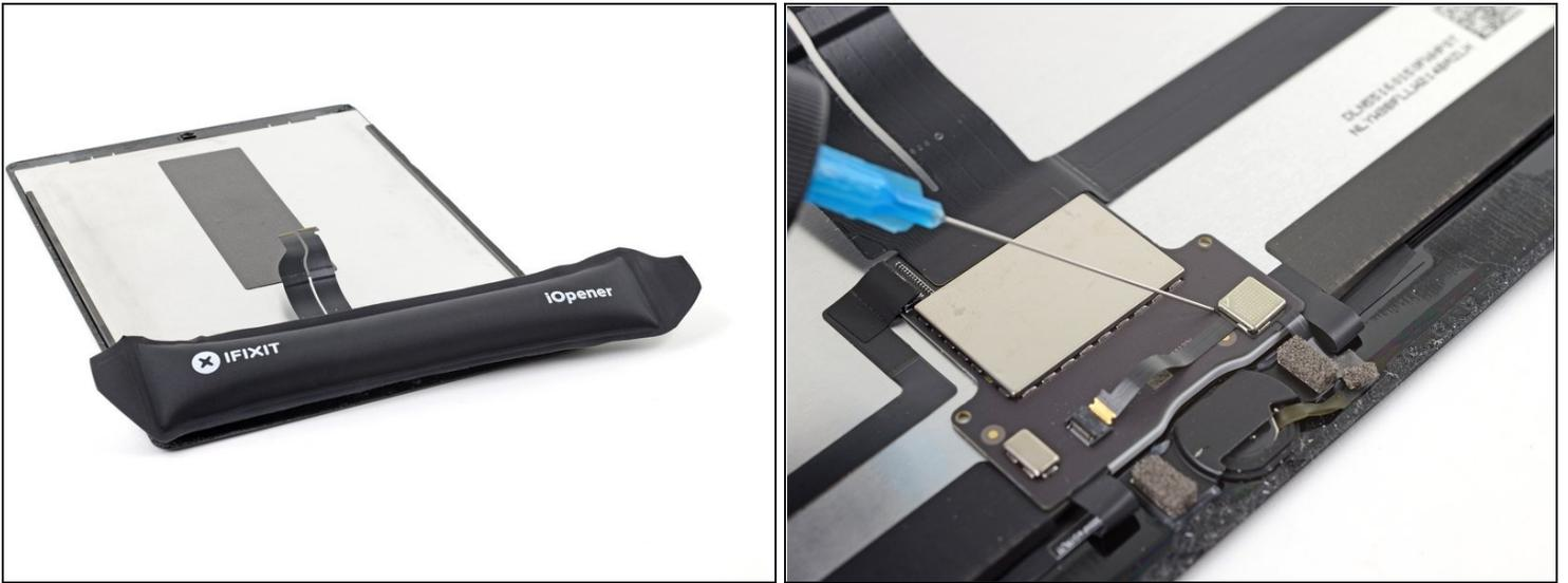
⚠ The home button's ribbon cable is **very** fragile. If it gets damaged, Touch ID will no longer function.
