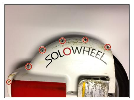
Using the Phillips screwdriver, remove the screws along the right side and handle on this side of the device.
