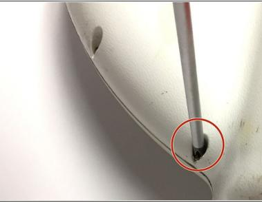
Using the Philips screwdriver, remove the 4 screws along the right side of the device.
