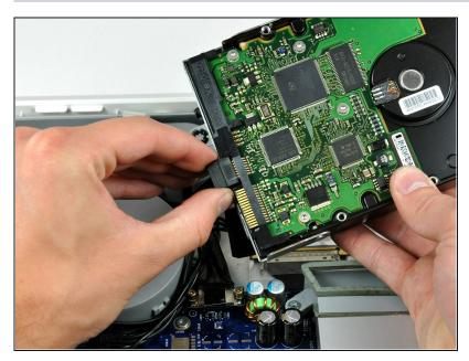
Pull the SATA data cable connector away from the hard drive. To reassemble your device, follow these instructions in reverse order.
