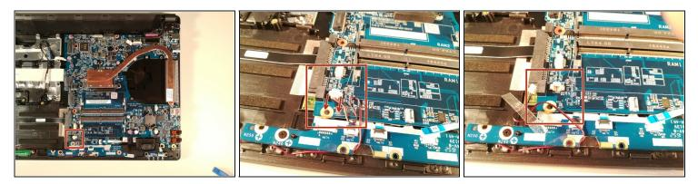
• Disconnect the connector marked in red by pulling it in the direction of the red arrows
