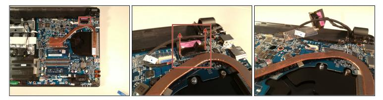
Disconnect the connector marked in red by lifting it up
