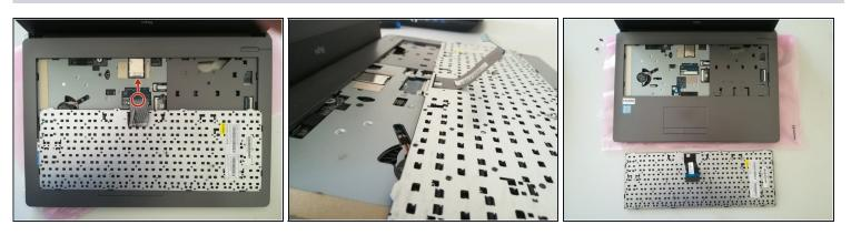
• Disconnect the connector circled in red in the direction of the arrow
