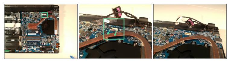
• Disconnect the connector marked in green by pulling it in the direction of green arrows
