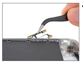
• Remove the dual microphone assembly.
