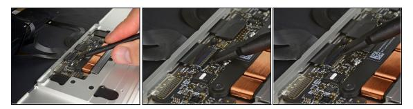
• Use a spudger to carefully flip up the retaining flap on the trackpad cable <u>ZIF connector</u>.
