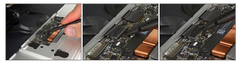
• Use a spudger to carefully flip up the retaining flap on the trackpad cable <u>ZIF</u> connector.
