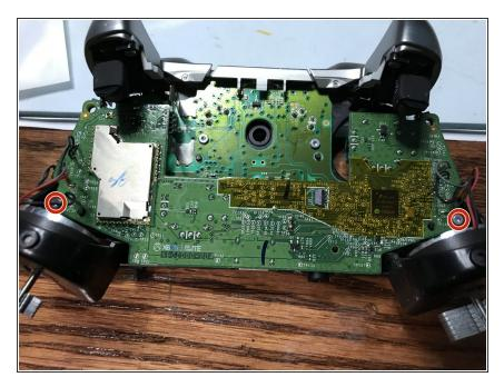
• Remove the 2 Torx (T6) screws
