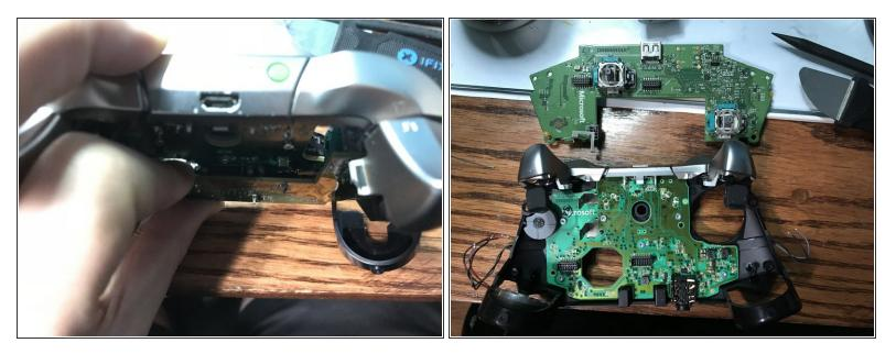
• Pull up from the "top" side of the controller on the sister board.
