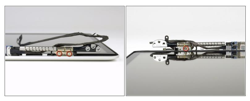
• Remove the three 5.2 mm T6 Torx screws securing the right clutch hinge to the display assembly.
