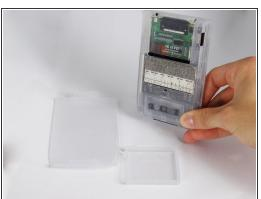
Slide the memory cartridge cover up and off the device.
