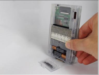
Remove the battery cover by releasing the clip from the main body of the device.
