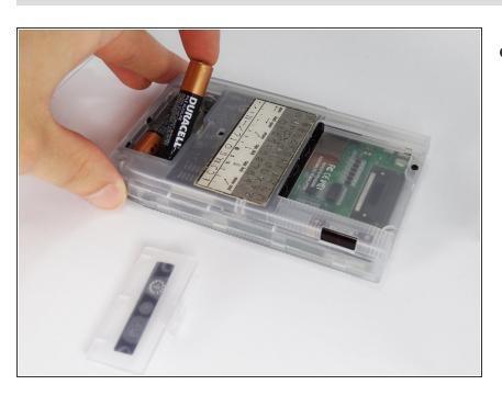
Remove the batteries from the device.
