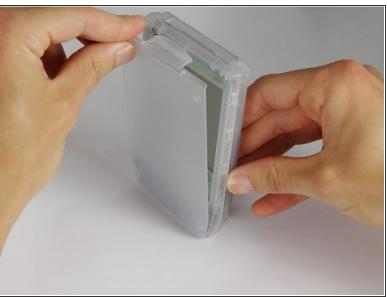
Remove the outer screen cover by releasing the top clip from the main body of the device.
