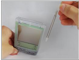
Pull out the stylus from the top right corner of the device.
