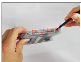
• Use the spudger to pry open the casing by applying pressure at 4 clips on both sides of the device.
