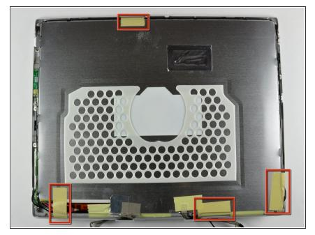
Remove the pieces of readily removable tape from around the perimeter of the display.
