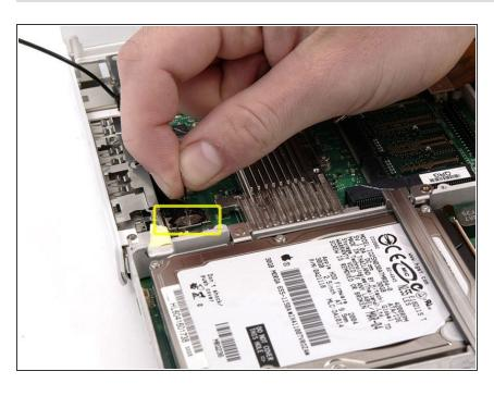
Use the black plastic handle to disconnect the display data cable from the logic board.
