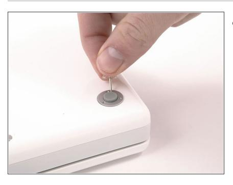
Use a pin (or anything you like) to remove the three rubber feet from the lower case.
