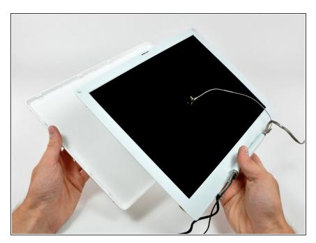
Lift the rear bezel off the display.
