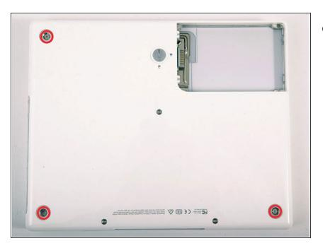
Remove the three newly-revealed Phillips screws.
