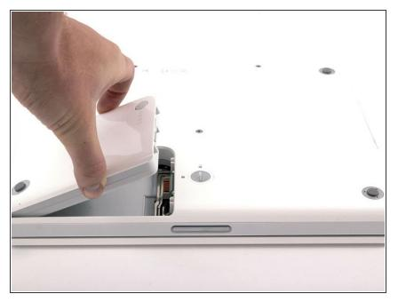
Lift the battery out of the computer.
