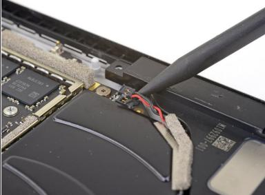
Use the point of a spudger to lift the right speaker connector out of its socket on the motherboard.
