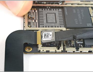
Use the flat end of a spudger to pry the display interconnect cable straight up and out of its socket on the motherboard.
