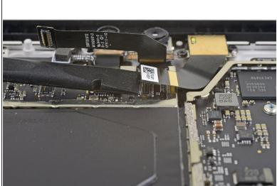
• Use the flat end of a spudger to pry the rear-facing camera connector up and out of its socket on the motherboard.
