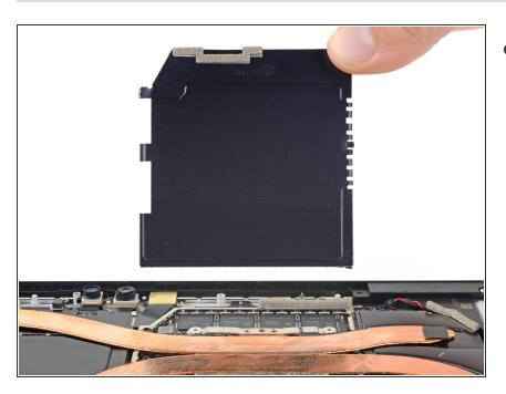
Remove the heat sink shield.
