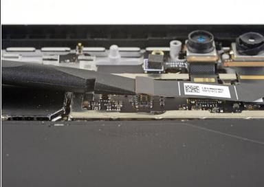
• Use the flat end of a spudger to pry the front-facing camera connector up and out of its socket on the motherboard.
