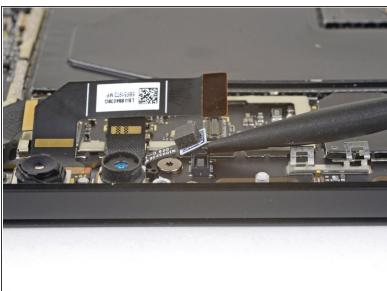
Use the flat end of a spudger to pry the microphone connector up and out of its socket on the motherboard.
