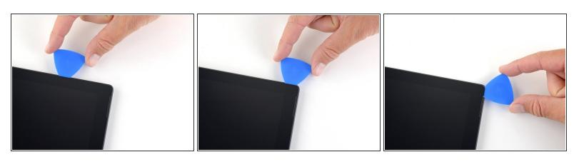
Once you cut the adhesive over the antennas (8.5 inches, or 22 cm, away from the left edge), slide the pick the rest of the way along the top edge of the surface and round the top right corner to slice through any remaining adhesive.
