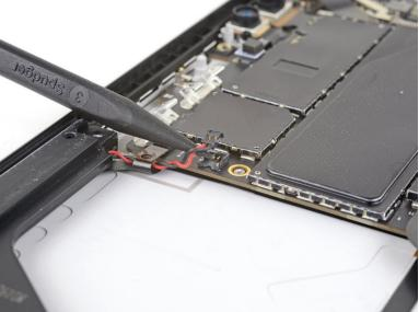
• Use the point of a spudger to lift the left speaker connector out of its socket on the motherboard.
