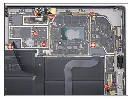
Use a T3 Torx driver to remove the eight 2.5 mm screws securing the motherboard.
