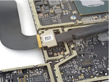
Use the flat end of a spudger to pry the digitizer connector straight up and out of its socket on the motherboard.
