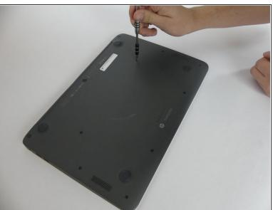
With the Phillips #00 screwdriver, remove the remaining eight 6mm screws. You will now have thirteen 6mm screws removed from the case.
