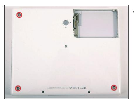
Remove the three newly-revealed Phillips screws.
