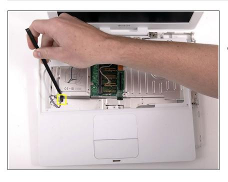
Lift the upper case off completely and disconnect the multicolored speaker cable from the logic board.
