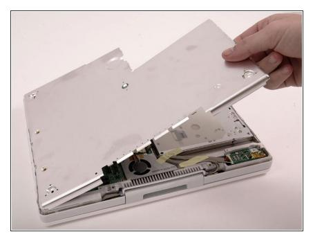
Lift the bottom shield off.
