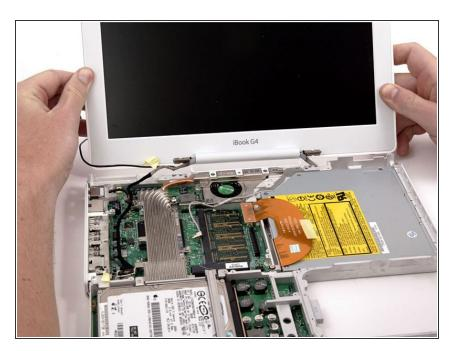
Tilt the display back, freeing it from the two metal alignment posts holding the hinges in place, and slide it away from you.
