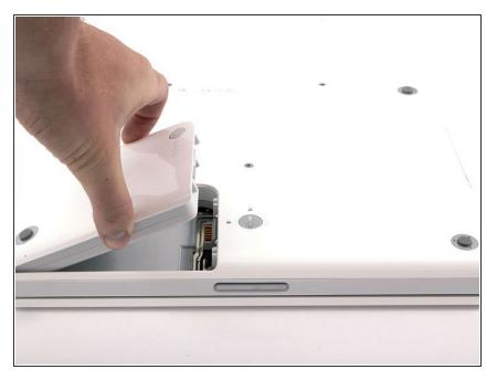
Lift the battery out of the computer.
