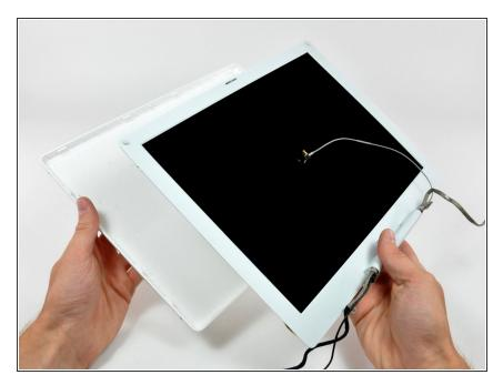
Lift the rear bezel off the display.
