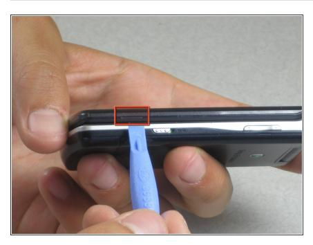
Find the small notch on the side of the phone. The notch is located by the "fast-forward" button and the "lock" switch.
