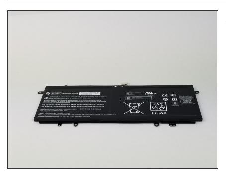
Carefully lift the battery and remove it from the device.
