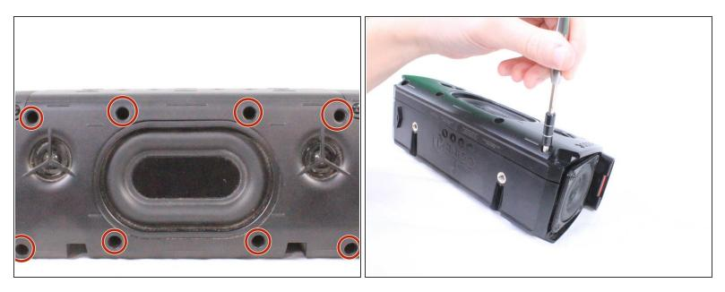
Using a #2.0 Hex screwdriver to unscrew the 8 12mm screws depicted.
