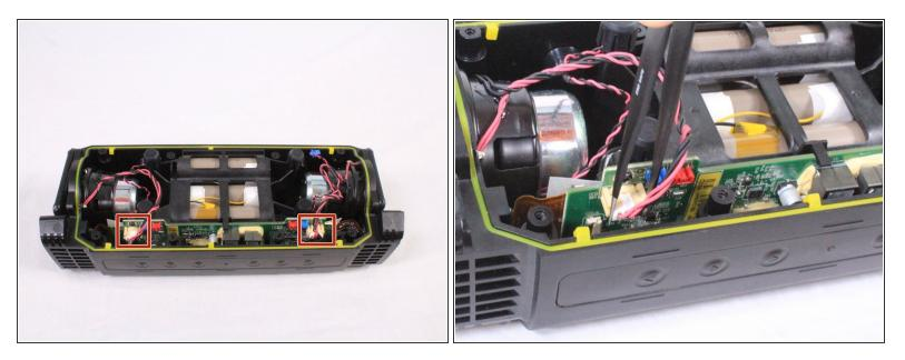
• Carefully untangle and remove the white bundled cable connectors from the motherboard.
