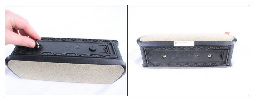
• Using your hand, unscrew the large screws underneath the speaker.
