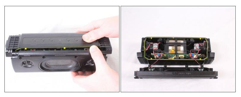
• Gently pull apart the front casing from the back casing.
