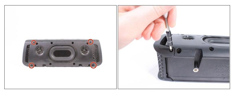
There are 8 screws (4 on each side) holding covers that conceal the bass speakers. Remove these 3mm screws using a #2.0 Hex screwdriver.
