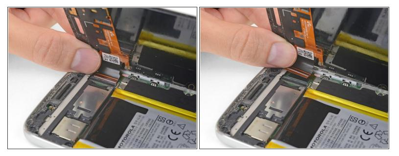
Gently pull the display cable to slide it out of its socket on the motherboard.
