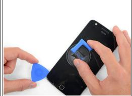
Slide the tool all along the left edge of the phone to slice through the adhesive securing the display.
