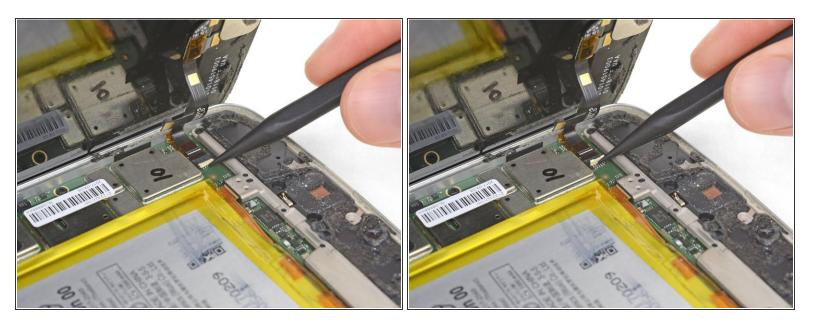
While holding the display open, use the point of a spudger to pry up the locking tab on the fingerprint sensor cable's <u>ZIF connector</u>.
