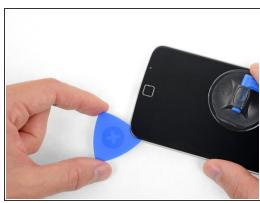
Continue separating the glue underneath the rest of the lower bezel.
