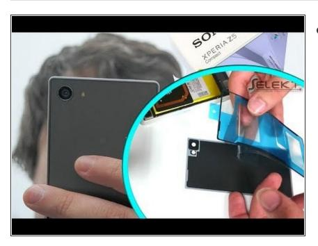
The one and only proper solution for sticking back cover in Xperia Z5 which keeps the water resistance.
