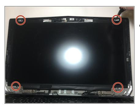
No you will unscrew the 2mm screws on the top and bottom side of the screen.
