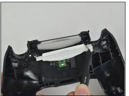
• Grip the right hand corner of the opaque white piece with a pair of tweezers, and pull it upwards to remove it.
