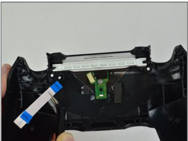
• Pull the ribbon cable from the charge port, using a set of tweezers.
