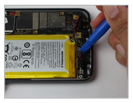
Using the plastic opening tool, unplug the oscillating vibration motor.
