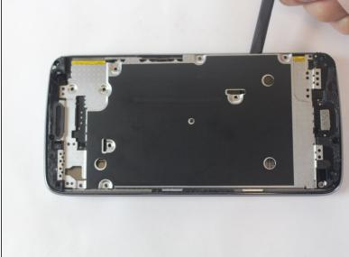
Remove the interior metal covering using the plastic opening tool.
