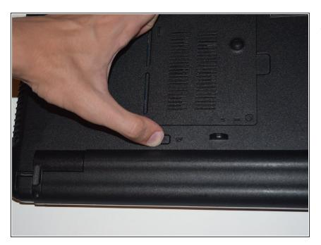
Unlock the battery by pushing and holding the lock button.
