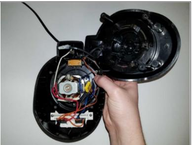
Remove the back panel using a Phillips #1 Screwdriver on the four screws that hold it in place.
