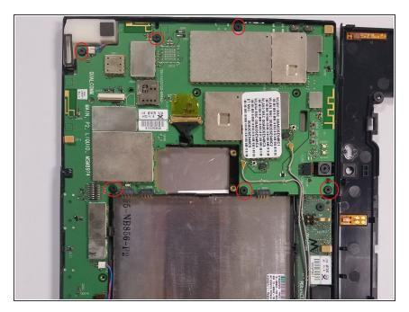
Using the Phillips PH1, remove all 6 of the 3x2.5mm screws (circled in red) holding the motherboard in place.
