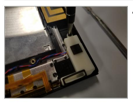
Use the Phillips PH1 screwdriver to remove the 3x2.5mm screw on the right speaker.
