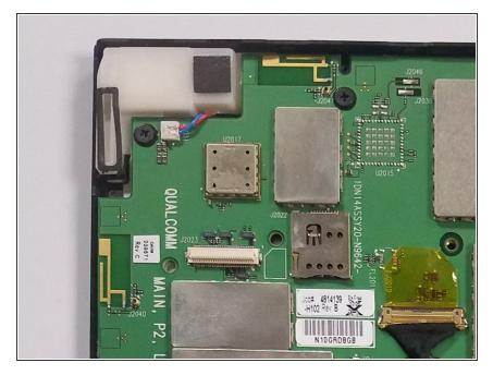
Locate the two speakers in each of the bottom corners (left and right).
