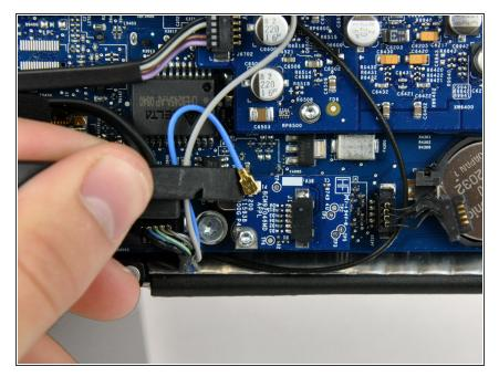
• Use the flat end of a spudger to pry the bluetooth antenna connector up off the bluetooth board.
