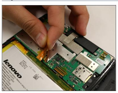
Gently detach the connector from the motherboard by pulling up on it.
