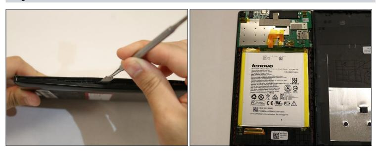
• Starting at any point along the seam of the case carefully pry it open with the metal spudger, slowly working your way around the outside until the case can come apart.
