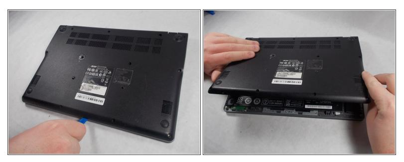
• Pry the back panel open with the plastic opening tool.
