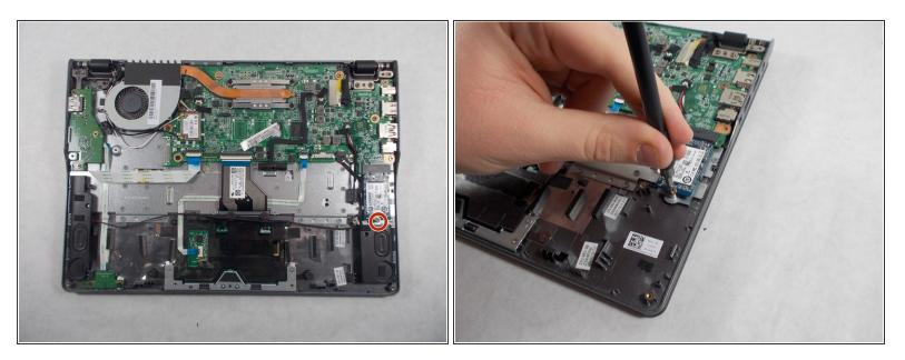
• Remove the single 3.0mm screw securing the solid state drive using a Phillips #1 screwdriver.
