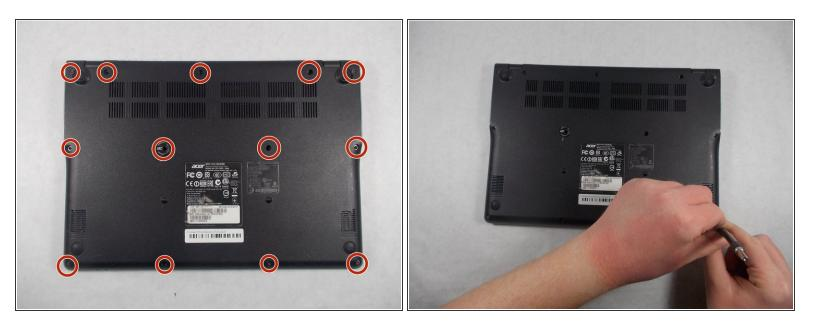
• Remove the thirteen 6.0mm screws on the back panel using your Phillips #1 screwdriver.
