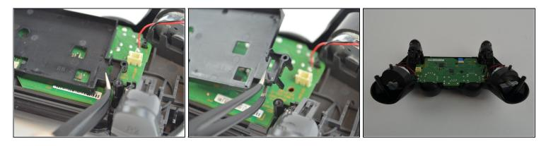
• Unhook the battery case from the motherboard, and pull it off.
