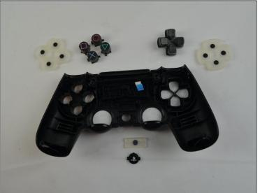
• Remove the old buttons, and replace them with new ones using a pair of tweezers.
