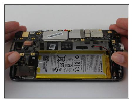
Remove the motherboard from the phone by prying it up with the plastic opening tool.
