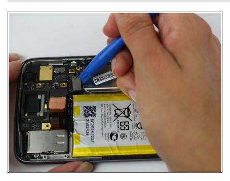
Unplug the flat-top connector with the plastic opening tool.
