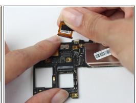
• Release the ZIF connector and remove the camera from the board.
