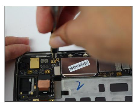
Using the Philips 000 Screwdriver, unscrew the 3.1 mm screw.
