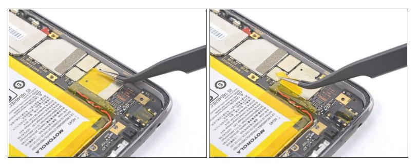
Remove the yellow tape covering the battery connector.
